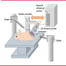
Detail from Figure 1, *Parasaram V. et al*, 2022. Design of our 3D-vibrational shear wave elastography (3D-VSWE) platform: schematic of the apparatus used to acquire VSWE data.
