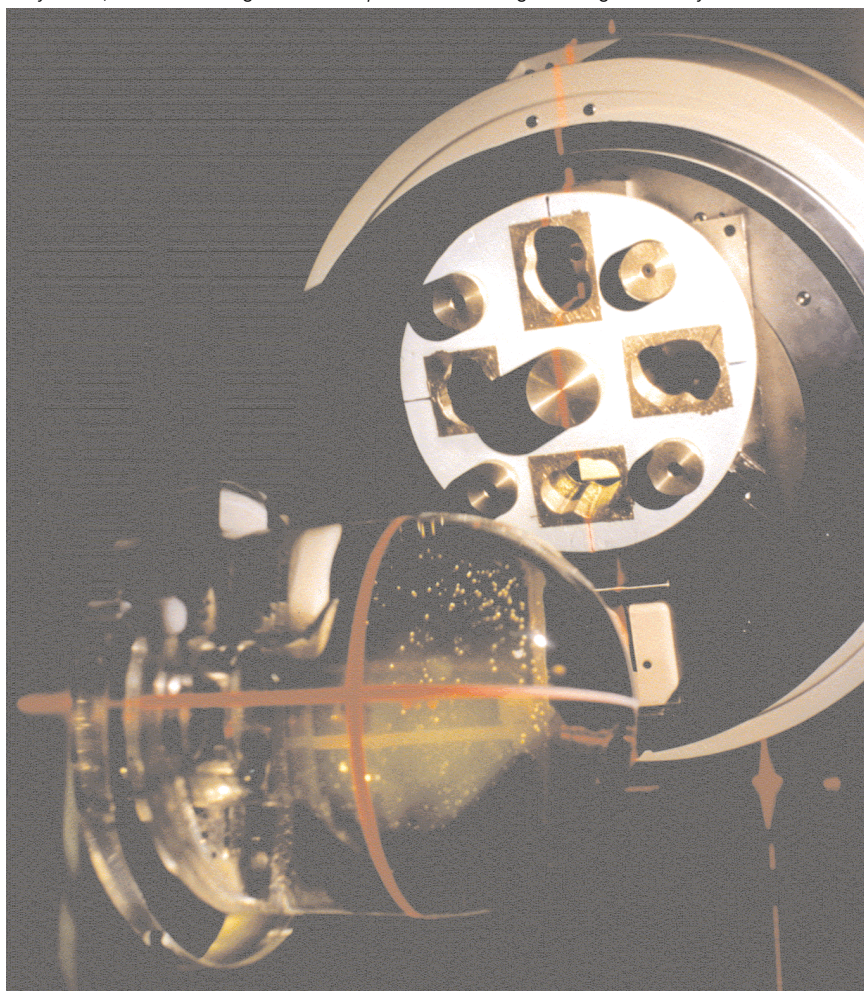
Figure 2 A conformal carousel mounted on a linear accelerator head for shaping a patient's set of four 6MV X-ray beams, shown here being checked on a phantom containing a BANG gel dosimetry insert
